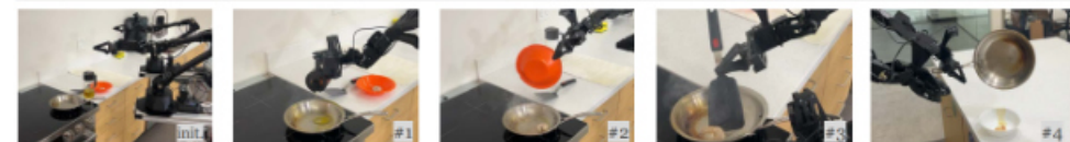
Cook Shrimp: The robot is randomized up to 5cm and all objects up to 2cm. The right gripper first pours oil into the hot pan (#1) followed by raw shrimp (#2). With left gripper lifting the pan at an angle, the right gripper grasps the spatula and flips the shrimp (#3). The robot then turns around and pours the shrimp into an empty bowl (#4) before placing the pan on the table. Each demo has 3750 steps or 75 seconds.
