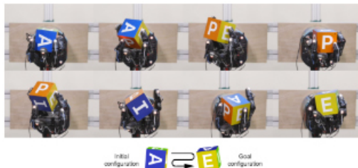
Figure 1: A five-fingered humanoid hand trained with reinforcement learning manipulating a block from an initial configuration to a goal configuration using vision for sensing.
